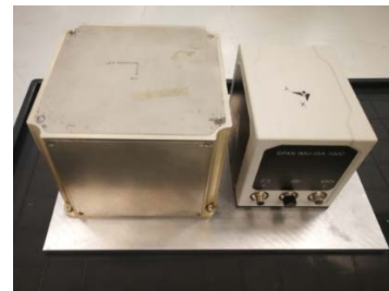
Figure 5-3: ALBATROS system and ISA-100C IMU fixed to the common mechanical fixture
