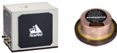
Figure 5-1: ISA-100C positioned in the left whereas HG1700 IMU is located in the right
